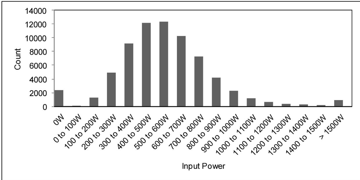
**Figure 1 - Metered Power Supply Input Power Distribution**
