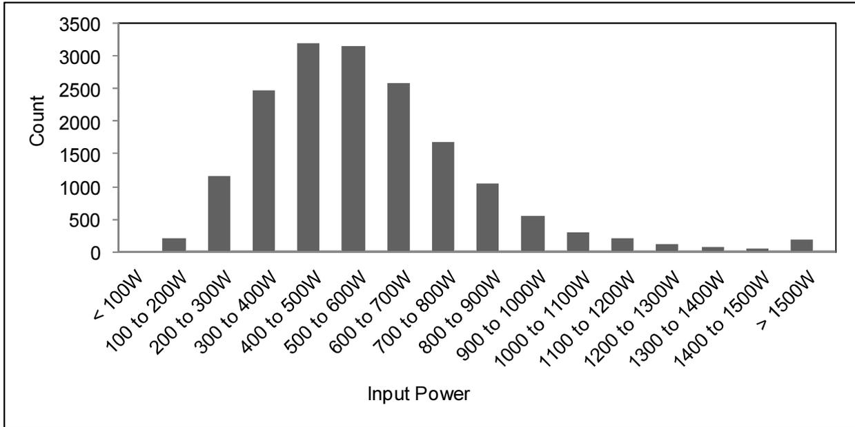
**Figure 5 - Sample System Power Supply Load Distribution**
