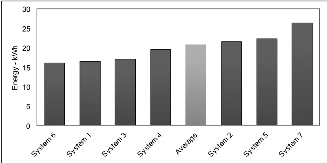
**Figure 8 - Critical Facility Energy Requirements per Subscriber**
