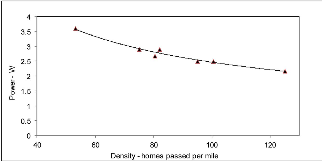
**Figure 10 - Access Network Powering Requirements**
