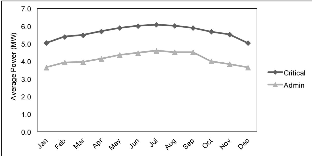
**Figure 2 - Sample System Facility Average Load Profile**
